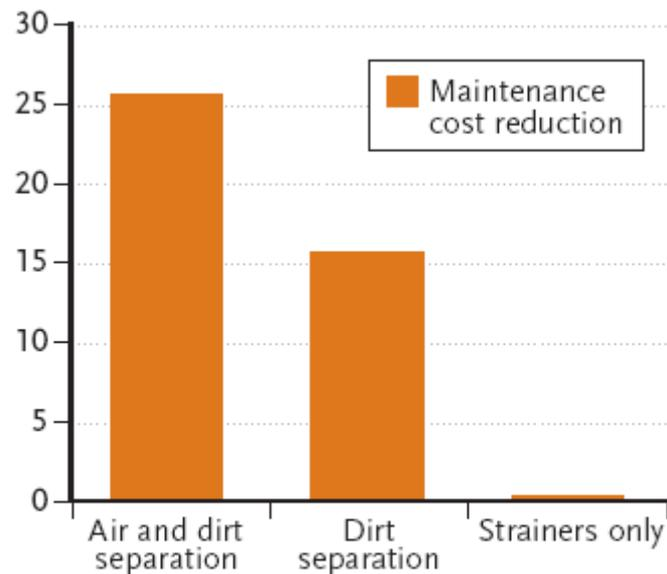
Figure 6: Case study one – impact of deaerators and dirt separators on maintenance costs
