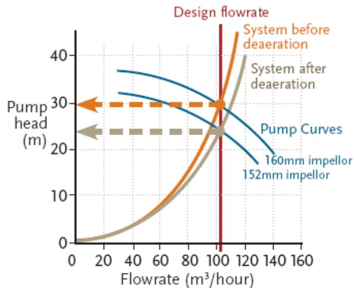
Figure 7: Case study two – pump power reduction through deaeration
